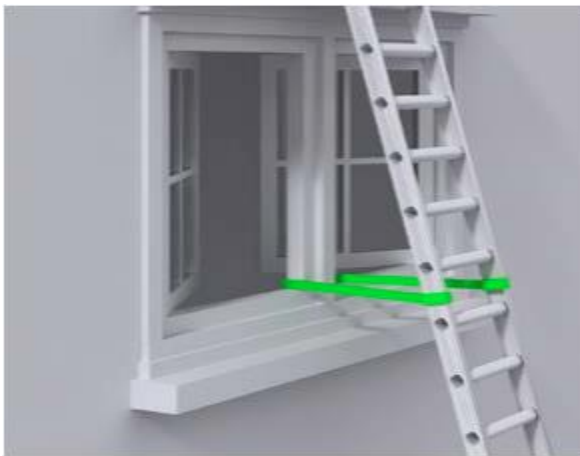
Figure 7 Correct – tying part way down
