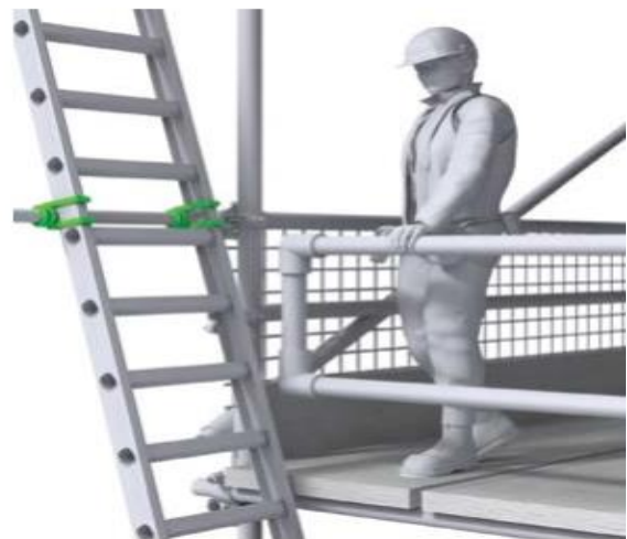
Figure 9 Correct – access ladders should be tied and extend at least 1 m above the landing point to provide a secure handhold
