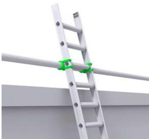
Figure 6 Correct – ladder tied at top stiles (correct for working on, but not for gaining access to a working platform/roof etc)
