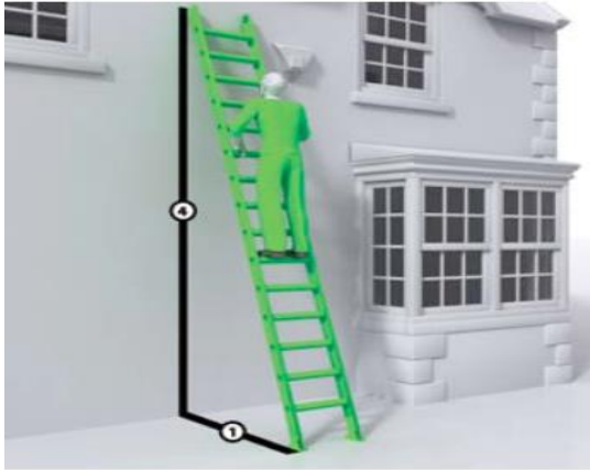
Figure 1 Ladder showing the correct 1 in 4 angle (means of securing omitted for clarity)
