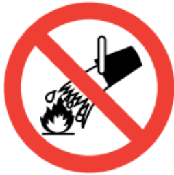
Do not extinguish with water
