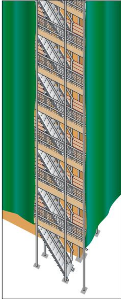
Figure 5 Where sheeted scaffolds form part of the escape
