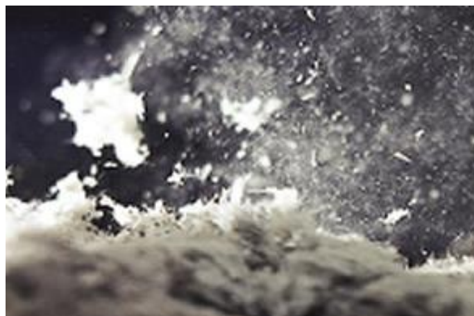
Release of loose fill asbestos fibres
